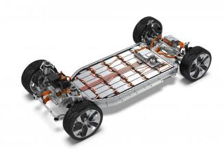
of a pack is given by the number of kilowatt-hours (kWh) of energy that it can hold. A typical EV pack might hold 60-150 kWh. Some packs are air-cooled while others are liquid-cooled. Battery packs are extremely heavy (well over 1,000 pounds) and are often placed low, under the vehicle floor, to produce a low center of gravity to enhance handling performance. The bigger the pack, the further you can go.
