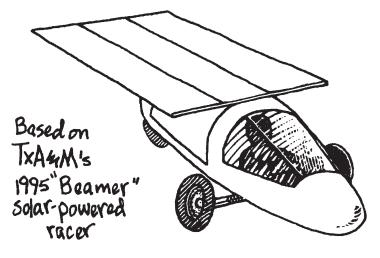
**POWERED BY THE SUN** A solar car has a solar panel that changes sunlight into electricity.
