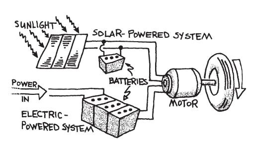
**SOLAR AND ELECTRIC-POWERED CARS** Sunlight or electricity can be used to power a car's motor instead of gasoline or diesel. If the car is driving fast, the motor uses all of the power from the solar panel. In some cases, the car may need more power than the panel can provide. Then the motor uses energy stored in the batteries.
